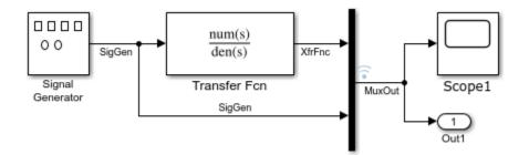
To complete the tutorial, you must already know how to create, configure, and simulate such a model. As you go through the tutorial, you transform slrt\_ex\_osc\_nrt into a Simulink Real-Time model configured to build as a real-time application. You then build, download, and execute the real-time application on your target computer.
